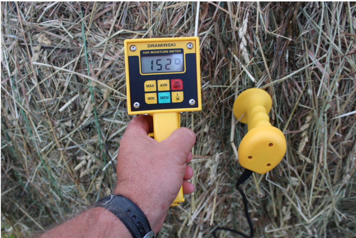
Figure 2. This hay was baled above the 18-20% moisture range and has reached an internal temperature of more than 150 degrees Fahrenheit. Heating damages protein making it unavailable to the animal. If stored in a tightly packed hay barn, this bale could start a hay fire.
