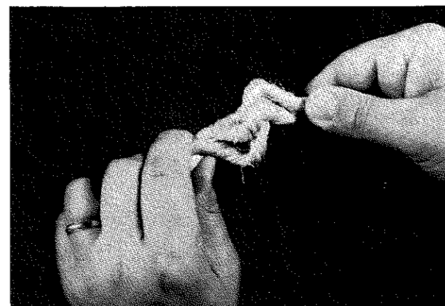
Figure 8. Take the whipped end of the rope in your left hand. Place your right hand about 3 inches from your left hand. Turn your left hand toward you and your right hand away from you so the rope twists open.
