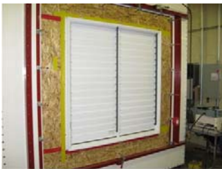
Figure 2 - Plastic shutter on test chamber
