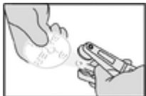
Figure 2 Slide tag under the clip of the pliers by depressing the lever.
